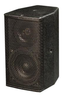
The EMS-51 is a compact, versatile, fill loudspeaker product designed for a wide variety of compact and discreet sound reinforcement applications. It features a high-power 5" (127mm) LF drive unit in an infinite baffle enclosure, and a 1.1" (28mm) soft dome high frequency drive unit. These components are matched by an internal passive crossover network for unprecedented sonic quality from a completely passive enclosure.
